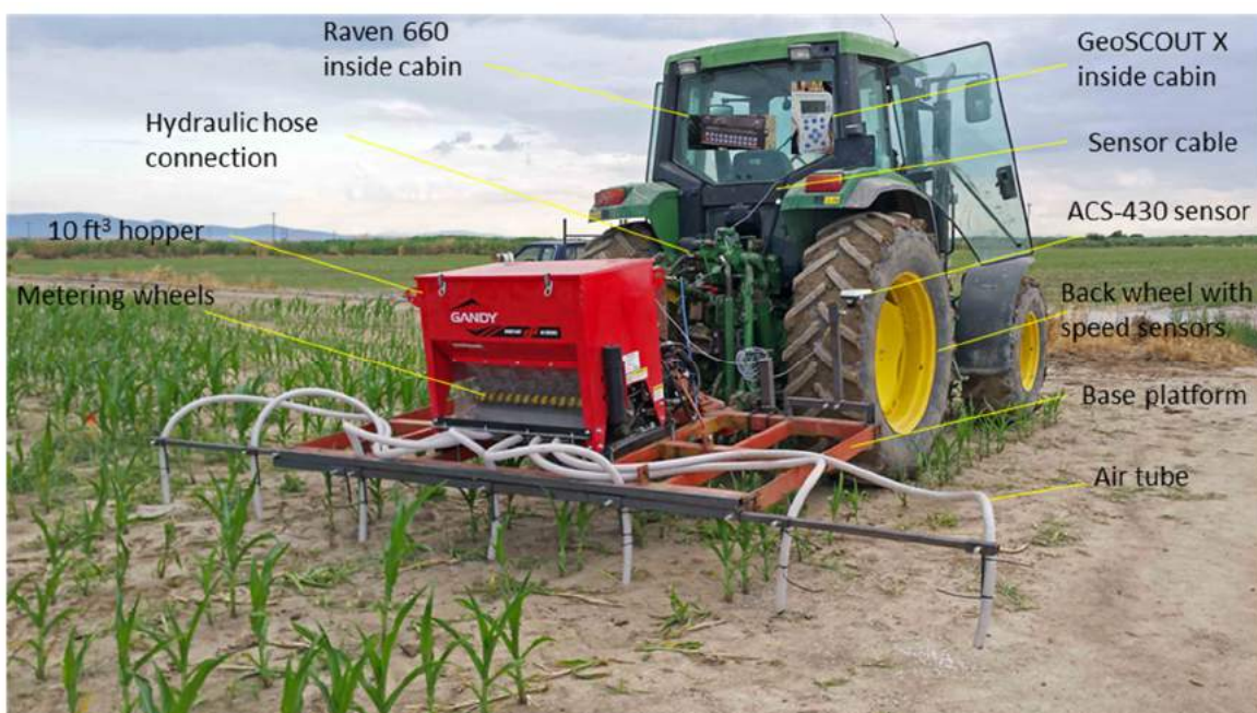
Figure 2. Various components of the VRT application system after installation
